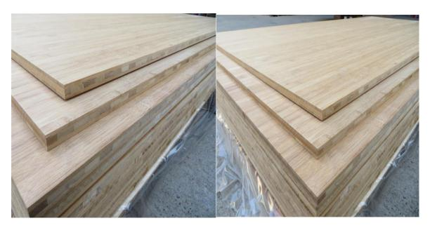
Bamboo plywood is especially interesting in those applications where the side of plywood remains visible, like steps of a staircase and kitchen work tops.
