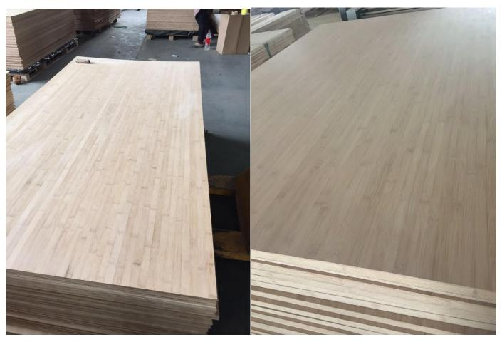
Bamboo plywood is made of fine layers of bamboo strips laying in parallel order.
